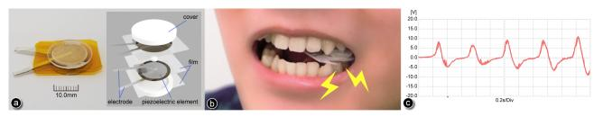
Figure 1. (a) Electric taste apparatus: Unlimited Electric Gum. (b) Image of a user chewing the apparatus. (c) Waveform of the piezoelectric voltage.
