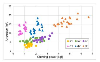
Figure 2. Amperage vs. chewing power (s1-3: one piezoelectric element, d1-3: two piezoelectric elements).
