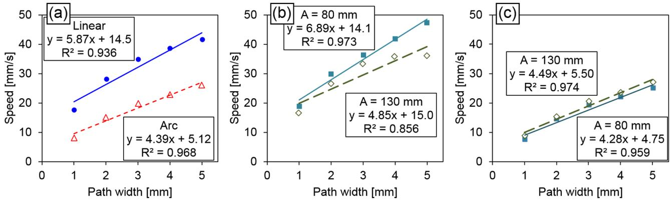
Figure 6. Speed versus path width. (a) Relationships for the linear and arc-like shapes, and relationships obtained by dividing two  $A$  values for (b) linear and (c) arc-like shapes.
