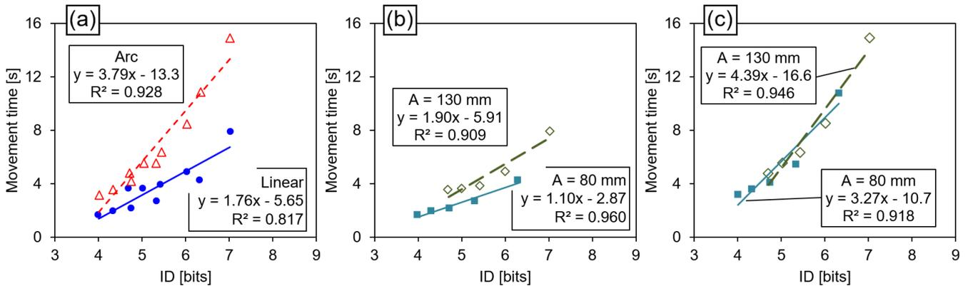
Figure 7. Movement time versus Fitts' index of difficulty. (a) Relationships for the linear and arc-like shapes, and relationships obtained by dividing two  $A$  values for (b) linear and (c) arc-like shapes.
