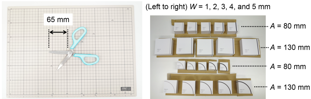
Figure 2. Scissors (left) and the pieces of paper used in the experiment (right).
