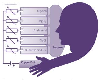
**Figure 4**: The system forms an electrical circuit together with the human body.
