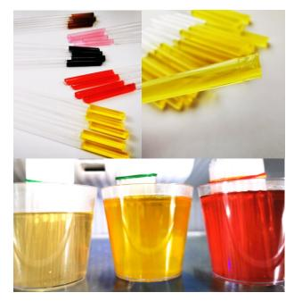
**Figure 2**: (Upper left) Five types of electrolytes dissolved and condensed into five gels, added food coloring. Brown gels are MgCl<sub>2</sub>, pink gels are glutamic sodium, black gels are NaCl, red gels are glycine, yellow gels are citric acid. (Upper right) The amount of gel exposure in contact with the tongue. (Below) Production process. We added solution to heated agar, inserted tubes, and chilled them in the refrigerator.
