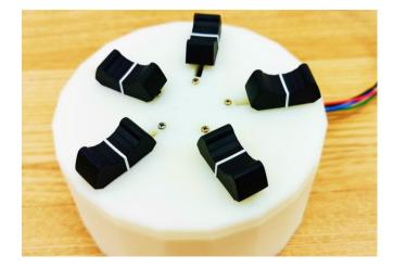
**Figure 3**: Controller. Variable resistors are connected to the ends of each of the five gels. It is shaped like a pentagonal radar chart of taste.
