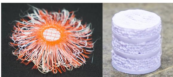
図8 造形中のレイヤ変更。(左) 3D printed hair [21]. (右) Expressive FDM [22].
