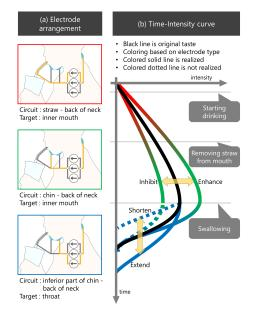
Figure 3: How we can control temporal change of taste using electrode arrangement. (a) Electrode arrangement (b) Time-intensity curve
