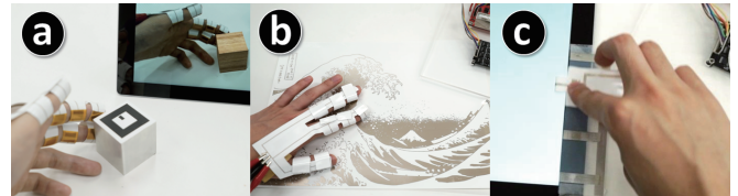
Figure 1. Printed tactile devices: (a) VR glove, (b) adding tactile feedback to a binarized image, and (c) tangible user interface with tactile feedback.
